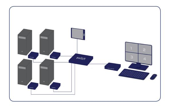
You can show, control and operate up to four different sources on one 4K screen.
