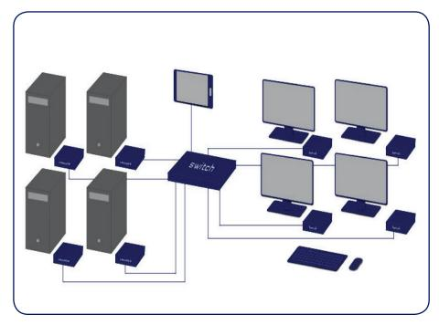
WITH ONE MOUSE AND ONE KEYBOARD YOU CAN OPERATE MULTIPLE MONITORS
